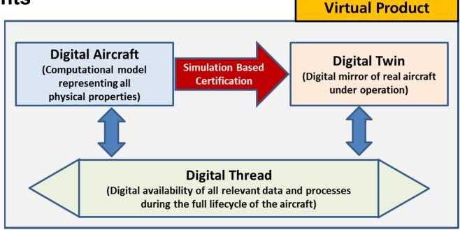
Digital Aircraft: Encompasses design, testing, manufacturing & certification process
