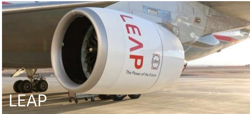
Next generation single aisle ... B737, A320 15% reduction in fuel burn (GE/Safran CFM56)
