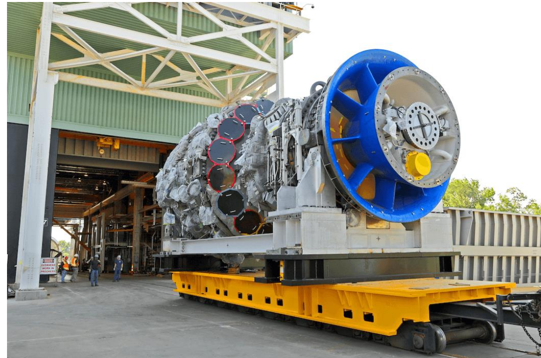
9HA.02 Gas Turbine Record setting 64% combined cycle efficiency @ 826 MW
