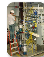
Lab-scale testing of novel CO 2 capture materials at NETL (<1 kW)
