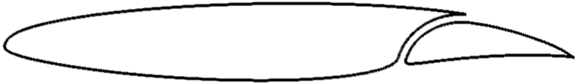
Figure 1.5: S207 Slotted, Natural-Laminar-Flow Airfoil Geometry
